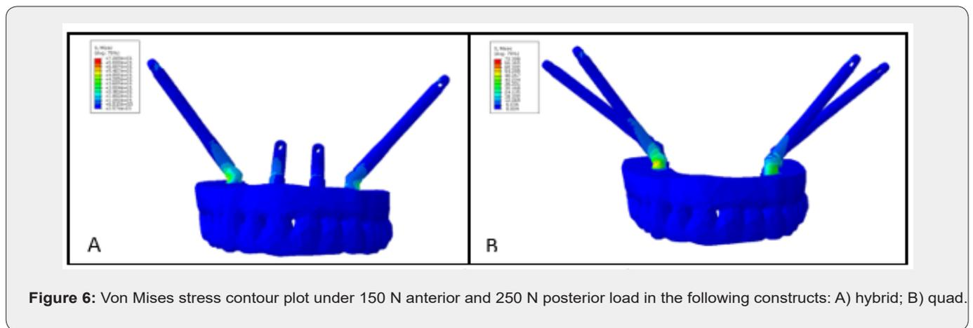
**Figure 6:** Von Mises stress contour plot under 150 N anterior and 250 N posterior load in the following constructs: A) hybrid; B) quad.
