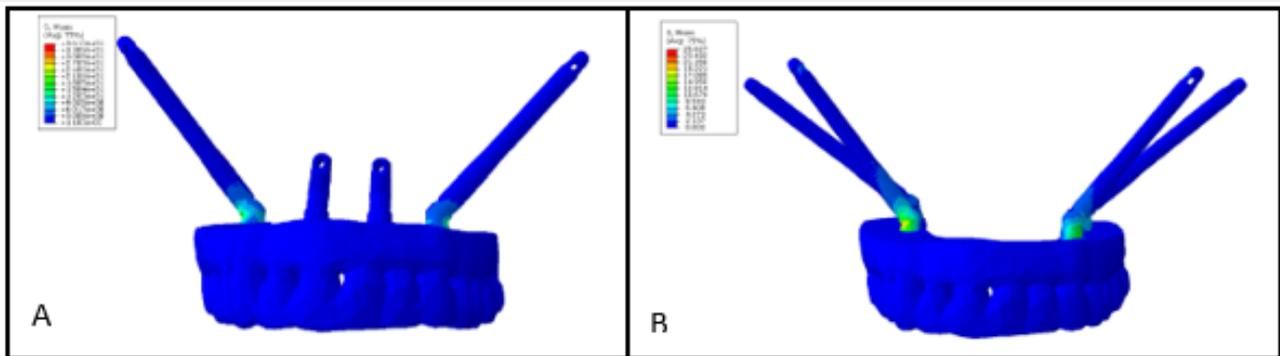
**Figure 5:** Von Mises stress contour plot under 150 N uniformly distributed load in the following constructs: A) hybrid; B) quad.
