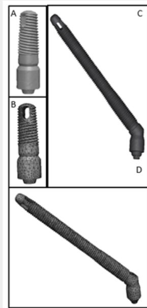
**Figure 4:** A) 3-D digital model of the traditional implant. B) Finite element model of the traditional implant. C) 3-D digital model of the zygomatic implant. D) Finite element model of the zygomatic implant.
