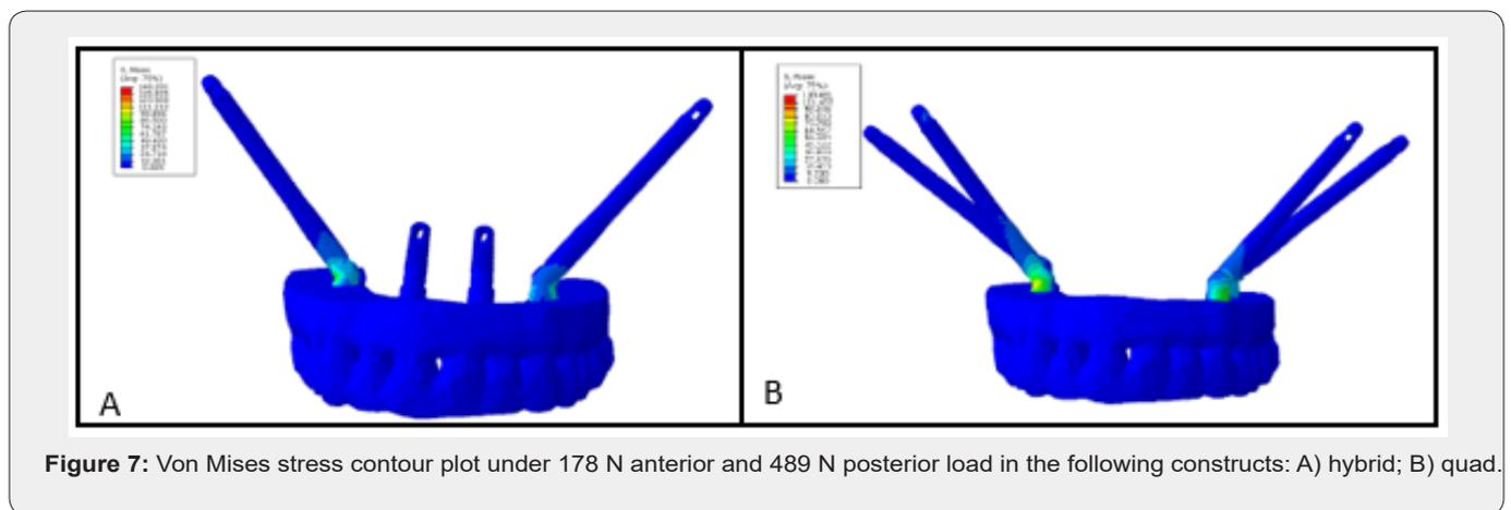
**Figure 7:** Von Mises stress contour plot under 178 N anterior and 489 N posterior load in the following constructs: A) hybrid; B) quad.
